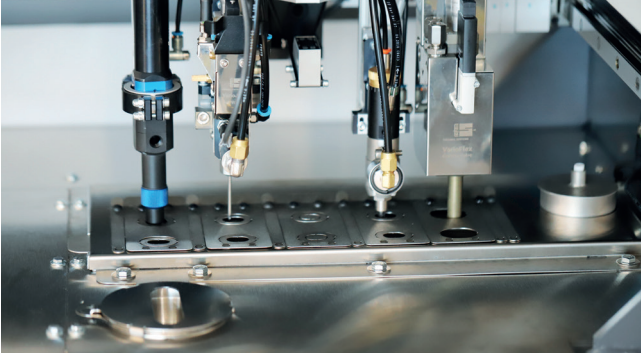
Brush and blowout station ProtectoXP
