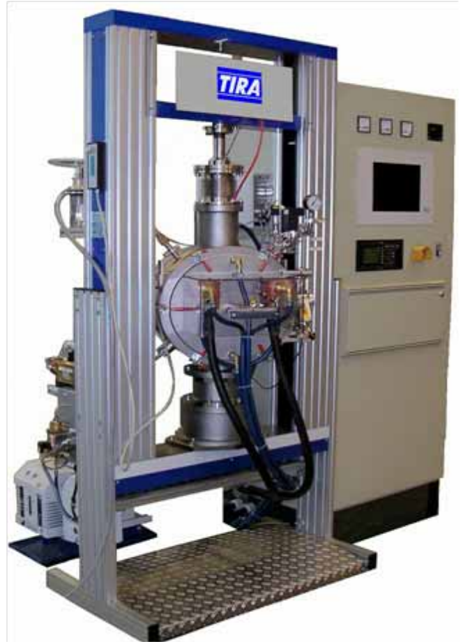
Flow limit determination TT 2820 with vacuum high-temperature kiln
