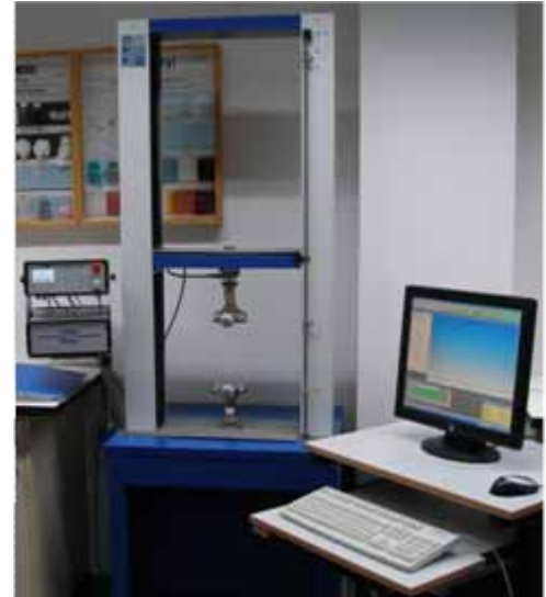
Tiratest 2410/20 Modernisation with external 1000 W output stage
