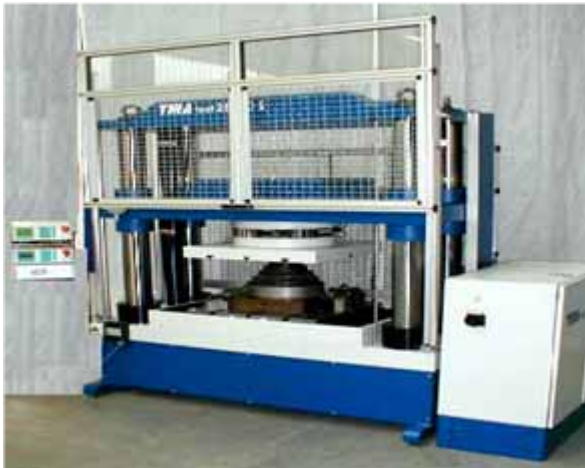
Examination of rubber springs from railcars TIRAtest 200 S
