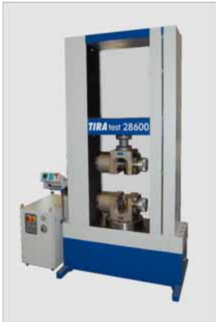
TIRAtest 28600 with hydraulic clamping tool
