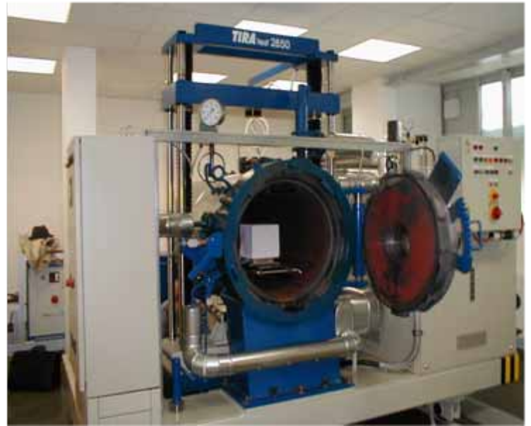
Examination of through-hardening of gas concrete by means of autoclaves to +150^{\circ}\text{C} / 50 \text{ bar} at Bergakademie Freiberg, Institute for silicate technology (Germany)
