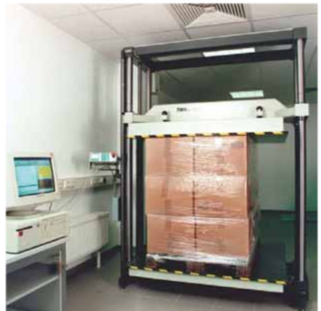
Testing of packaging material
