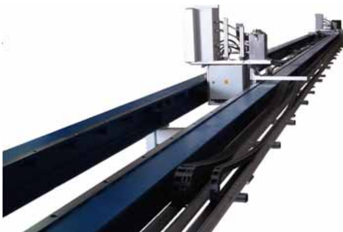
Wire testing machine up to 300 kN, travel 2 m, length 20 m
