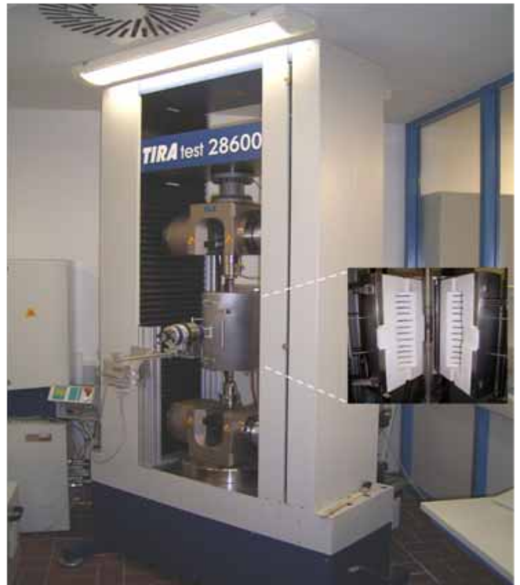
Retractable tube furnace up to +1100^{\circ}\text{C} including a high-temperature extensometer with 10 mm measurement path.
