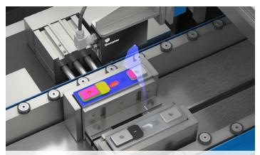
Gocator® 2530 inspecting battery weld
