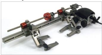
Needed to use the CHAIN Scanner as a mouse scanner with magnetic wheels holding the system instead of chain links.
